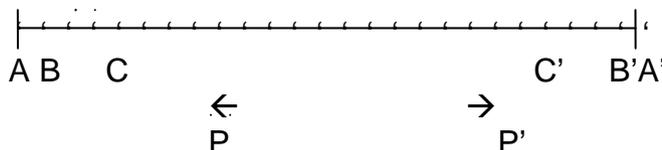
4) During the period CC' a pulse will show up a straight. During the periods BC, C'B' a pulse will show up nothing since the shorting of the inner brushes will "fill up" the input. But during the periods AB, B'A' a pulse would find open circuits and would show up a false straight.
