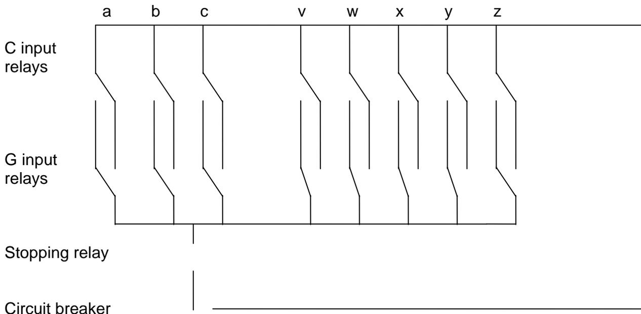
It will be seen in the diagram on page 5 of the previous note that the sensing relay associated with a current entry line is permanently down. Remember that the sensing relays are differential relays, which go up when current passes through one coil but not through the other.
